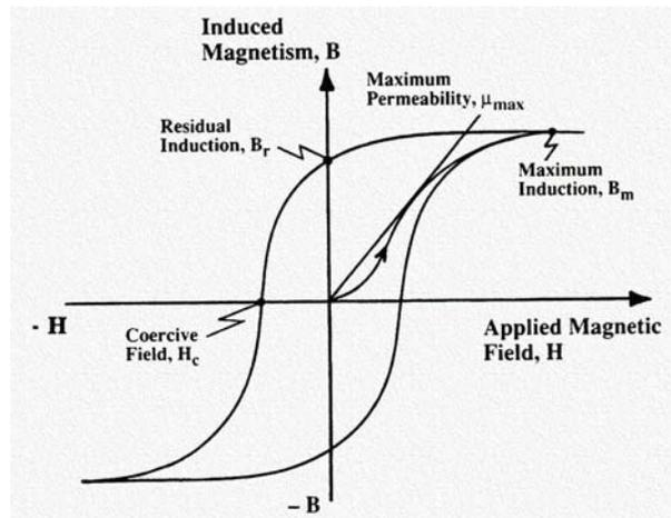
**Remanence or Residual Induction**,  $B_r$ , is the magnetic induction that remains after the magnetizing force has been removed.
